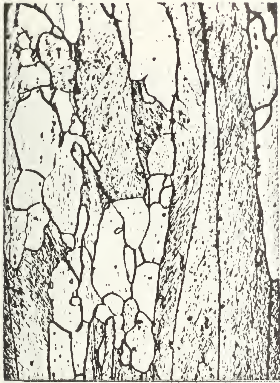
FIG. 20 AT 540°C FOR 18 MINUTES (ROCKWELL 30T 59.4)
